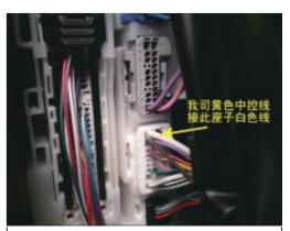
10. Find the central control under the ground wire. Our yellow color control wire is connected to the socket's white color wire.
