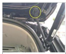
6. Remove the rubber plug of the original car and punch it with our drill bit. Our Hall wire passes through the rubber plug hole and goes to the tailgate cover.
