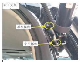
4. Remove the lower right bracket of the original car, install our lower right bracket (ball head facing inside the body) and electric pole, and fix it with the original car screws.
