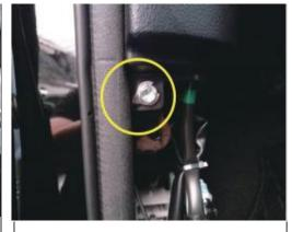
9. Locate the ground screw under the driver compartment and connect the ground wire.
