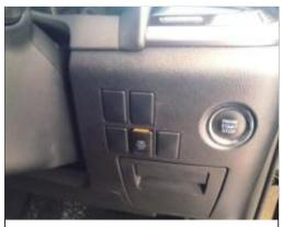
11. Remove the dummy button at the driver compartment according to the owner's habit, and install our front switch button.
