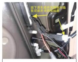
12. On the back of the original car tailgate opening button, find this socket and plug in our front switch adapter socket
