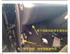
7. Find the power, ground and central control lines as shown in the co-driver compartment
