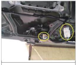
13. Locate the socket at the original door lock, unplug the original car socket and plug it into our three-way adapter socket.
