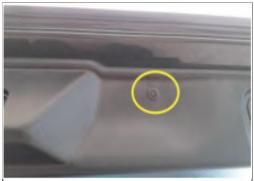
5. Remove the button of the original rear door and remove the trim
