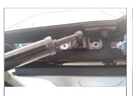
1. Remove the left support strut and left upper brackets of the original car, install our left upper bracket, and fix it with our screws.
