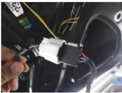
15. Unplug the original car socket at the door lock and insert it into our three-way adapter socket.
