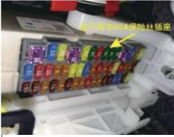
8. Remove the fuse cover as shown in the figure, unplug the original car 30A fuse, plug in our power socket
