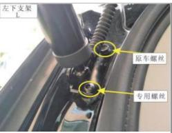
Remove the left lower bracket of the original car and install our left lower bracket (ball head facing inside the body) and our electric pole
