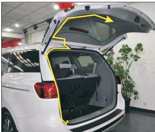
16. Electric door suction line go line to end cover plate
