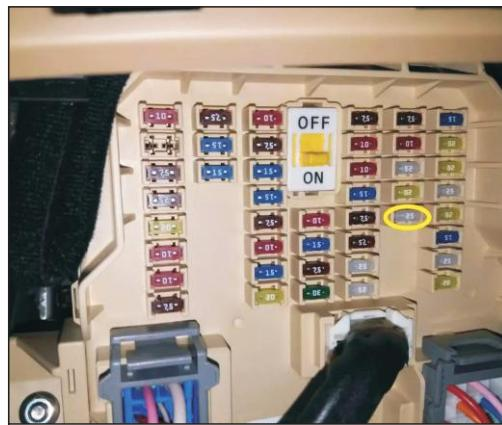
8. Remove the trim at the bottom of the main drive, unplug the original car 25 a fuse
