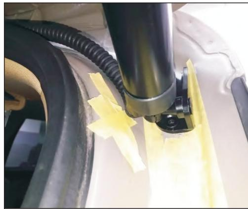
5. Remove the original car right bracket, we lower bracket, installation poles (the line ends of the poles down)
