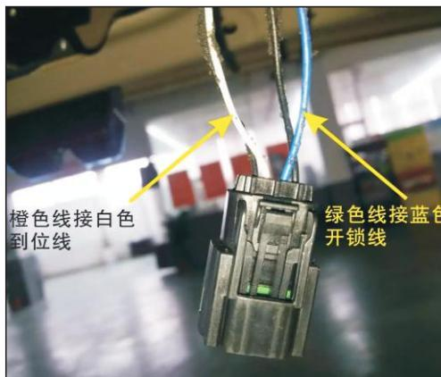
14. At the tail door locks unplug the saddle to take the orange line in the seat of the white line, green line after the blue line
