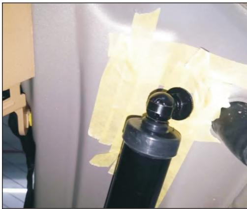
4. Remove the upper ball head, the original car installed at the upper ball head, the ball head and a gasket we deserve
