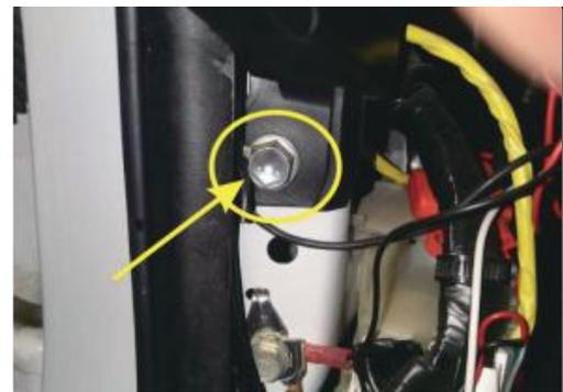
9. Remove the trim board at the side of the driver compartment, loosen the screw and connect the ground wire then tighten the screw.
