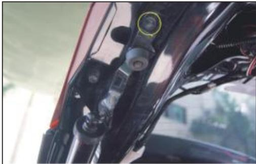
4. Install our electric pole with the upper bracket of the original car (the same steps are left and right)
