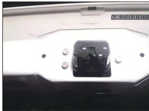
15. Remove the screw of the original car, remove the suction lock of the original car, install our electric suction lock, and fix it with the screw of the original car.
