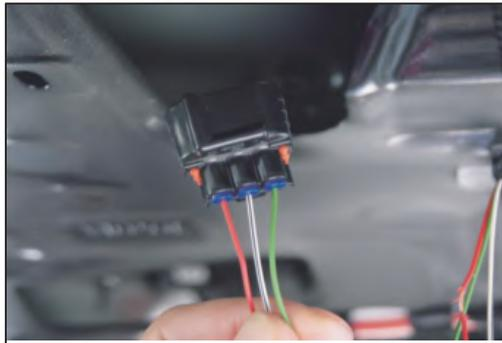
17. Connect the original car unlock plug directly with our provided three-way adapter socket, and plug the other end of our socket to the door lock socket.
