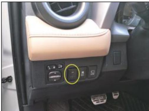
10. At driver compartment takes off the dummy button of the original car and install our front switch button.
