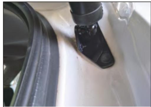
3. Remove the lower right bracket of the original car, replace with our lower right bracket of (ball head facing outward), and fix it with the original car screw.
