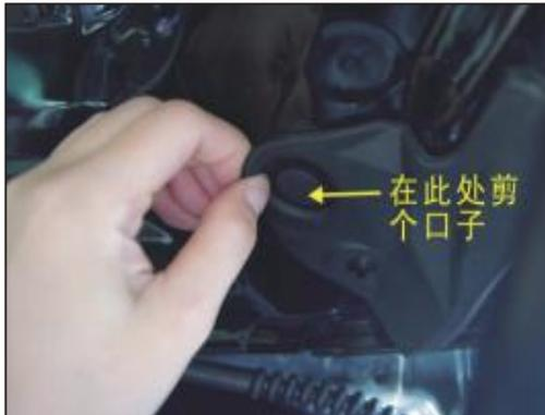
5. Remove the rubber stopper and cut a hole to facilitate Hall wire threading (the same steps on both sides)
