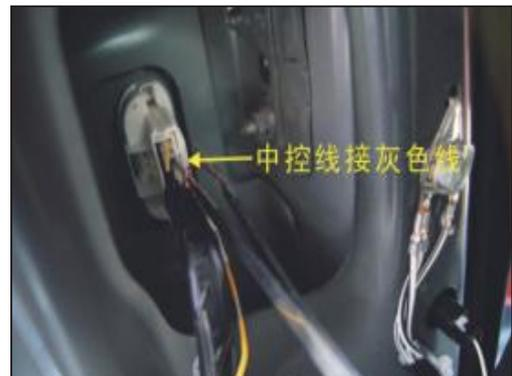
12. The central control wire is connected to grey color wire (the third hole in the second row from left to right)
