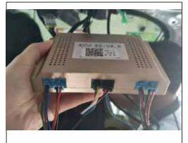
16. Hall wire, central control wire, power wire according to color insert one by one to control box
