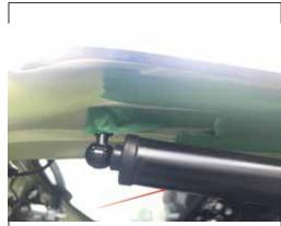
6. Install our right electric pole with the original car ball mount
