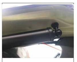
1. Remove the original car left support strut
