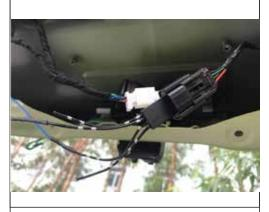
13. Connect electric suction lock plug to socket
