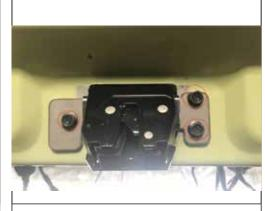
12.Remove the original lock and install our suction lock. Then, fixed with screw.
