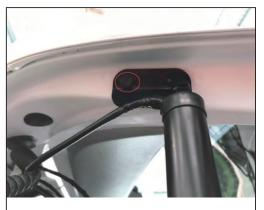
4.Remove the left upper ball head of the original car and install it. Our company specializes in it. The bracket is fixed with our screw
