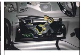
9.Remove the mechanical lock of the original car and install the tail door specially designed by our company Switch key, fixed with original screw
