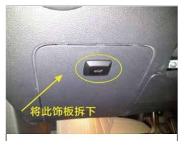
6. Remove the trim board under the main driving, find the power supply, remove the trim board, punch hole and install the front switch
