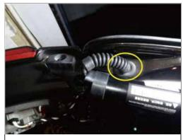
5. The electric pole Hall wire passes through the reserved hole and is plugged with rubber plug as shown in the figure (the left and right steps are the same)
