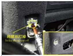
11. Remove the screw on the left side of the trunk and remove the button.
