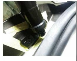
3. Remove the left lower bracket of the original car, install our lower left bracket, and fix the bracket with our screws.
