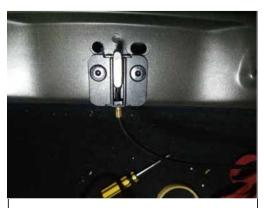
10. Remove the original car lock hook, install our electric suction lock hook, and fix it with our screws.
