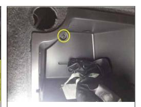
12. After knocking off the screw, the trim board is taken apart to facilitate the placement of our electric suction lock
