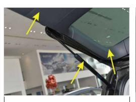
1. Remove the tailgate trim board and the original car support strut
