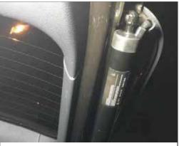
$2. \ \mbox{Install}$  our electric pole with the original car bracket (the left and right steps are the same)
