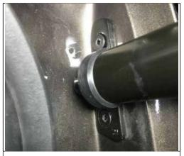
4. Remove the right lower bracket of the original car, install our lower right bracket, and fix the bracket with our screws.
