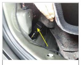
13. The electric suction lock is installed on the right side of the tailgate and fixed with our 3M glue (as shown in the figure)
